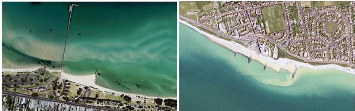
**For groynes to work as portrayed in Figure 5-3 of the EIA it would mean constructing these unchanging structures in a dynamic system while expecting sand to suddenly stop moving along the coastline - which is illogical. In fact, it is very likely that the construction of the groynes will reduce the accretion of sand downstream, exacerbating coastal erosion in other parts of the coastline.**
